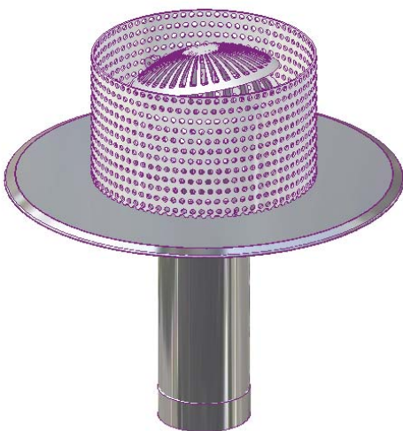
Optional T-12 Stainless Steel Ballast Guard on RD-14SS Roof Drain (Shown Friction Fitted To Drain Body)
