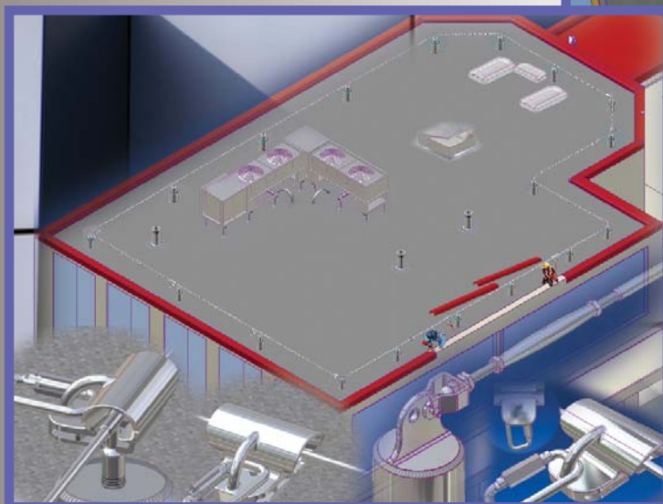
Illustration showing completion of roof edge using Thaler Horizontal Lifeline System (K-700 )
