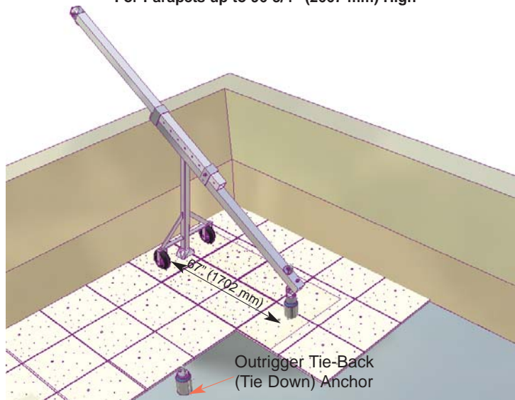
FARA-175-C PORTABLE OUTRIGGER BEAM For Parapets up to 60" (1524 mm) High
